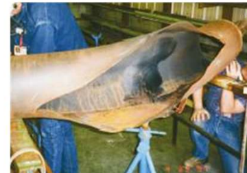
Failure in a high pressure extraction line at Fort Calhoun, 1997.
