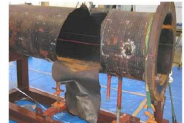
Failure in a main line in the condensate system at Mihama 3, 2004.
